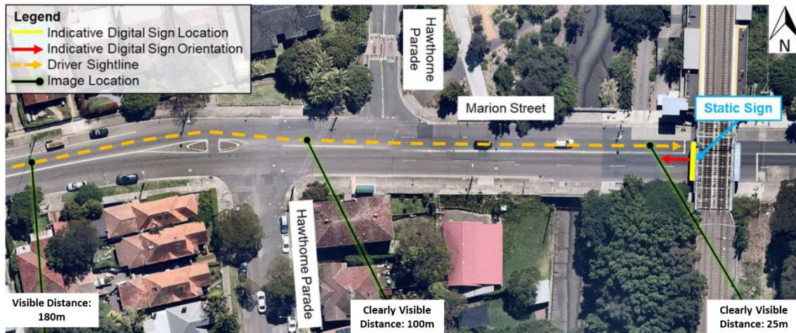
Figure 11: Signage exposure distance (Source: Bitzios Consulting)
